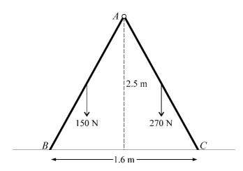
A step-ladder is modelled as two uniform rods AB and AC, freely jointed at A. The rods are in equilibrium in a vertical plane with B and C in contact with a rough horizontal surface. The rods have equal lengths; AB has weight 150 N and AC has weight 270 N. The point A is 2.5 m vertically above the surface, and BC = 1.6 m (see diagram).
